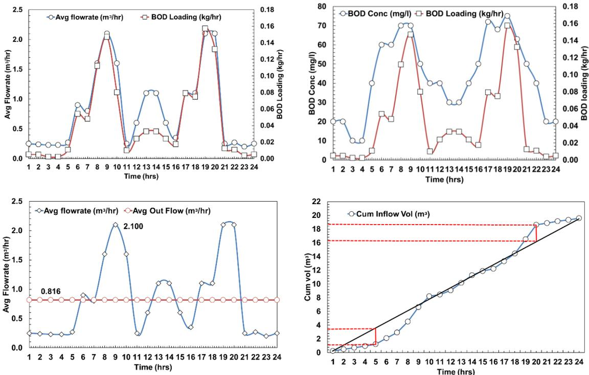
Fig. 2. Variation of BOD concentration, BOD loading, average flowrate, average outflow, cumulative volume of wastewater with time
