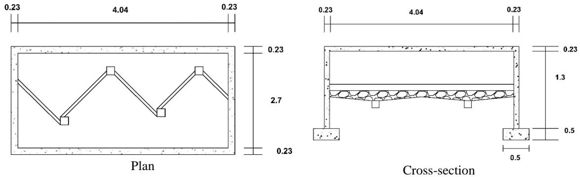
Fig. 6. Plan and Cross-section of designed Sludge Drying Bed (dimensions in m, not up to the scale)
