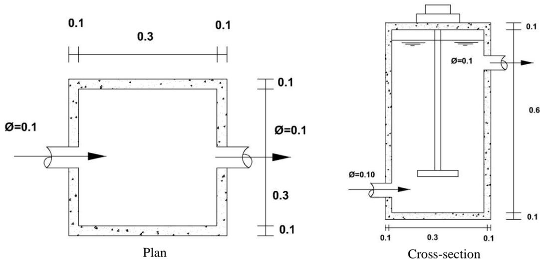
Fig. 4. Plan and Cross-section of designed Flash Mixer (dimensions in m, not up to the scale)
