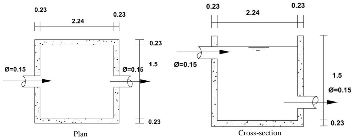
Fig. 3. Plan and Cross-section of designed Equalization Tank (dimensions in m, not up to the scale)
