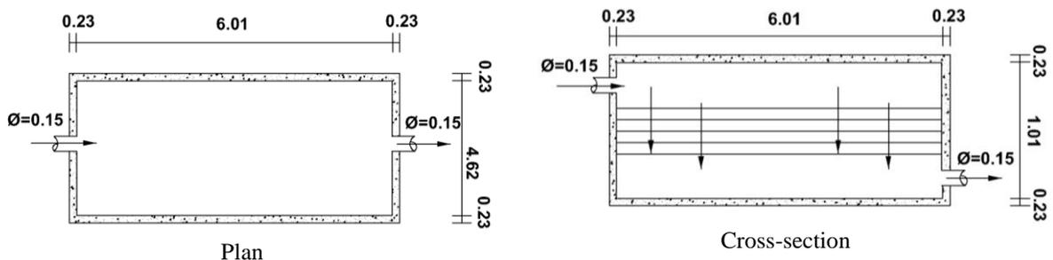
Fig. 7. Plan and Cross-section of designed Rapid Gravity Filter (dimensions in m, not up to the scale)
