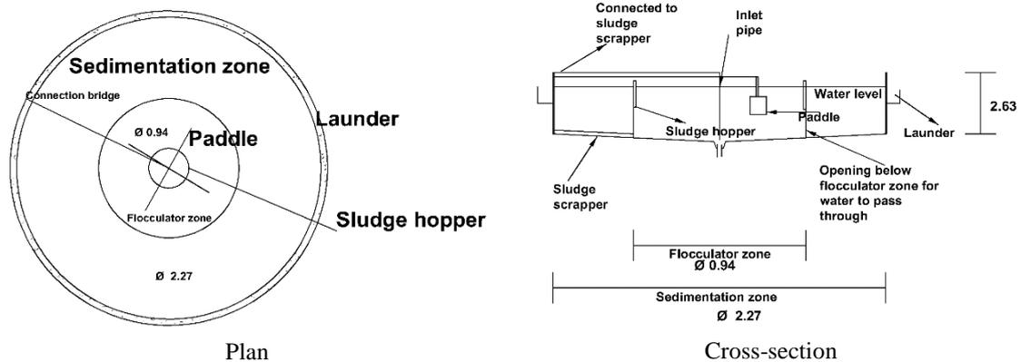
Fig. 5. Plan and Cross-section of designed Clariflocculator (dimensions in m, not up to the scale)
