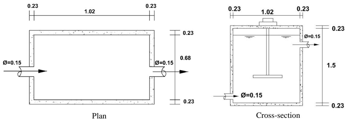
Fig. 8. Plan and Cross-section of designed Disinfection Unit (dimensions in m, not up to the scale)
